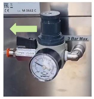
Turn the gas valve to *OPEN*, check that the pressure does not exceed 3 bar and switch the machine on.
