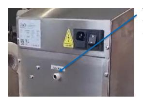
The gas cylinder must be attached to the gas inlet. Fit the gas cylinder onto the valve by turning it clockwise as far as it will go. Do not overtighten.
